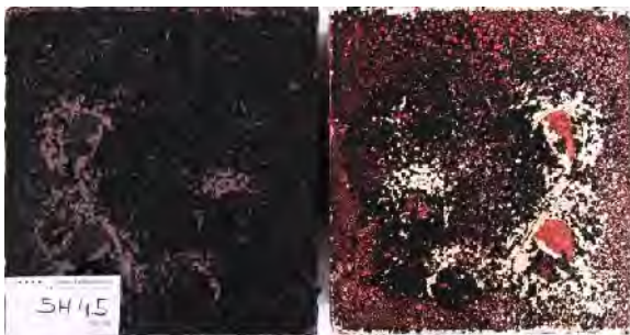
Figure 12: This test specimen has been cut open to display the clear blistering
