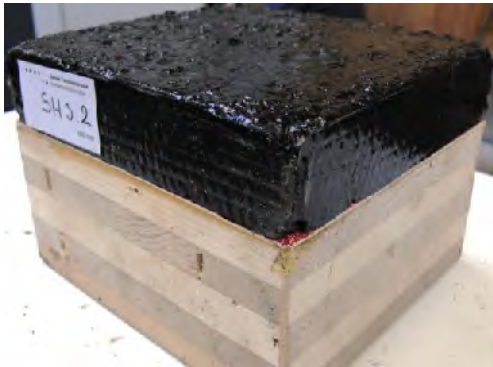
Figure 10: No blistering observed in this specimen of asphalt surfacing on CLT
