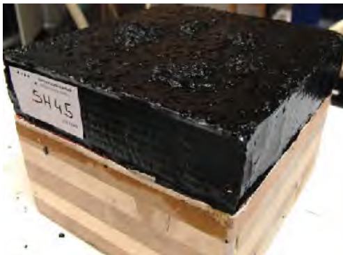
Figure 11: Clear blistering in the surfacing of this specimen of asphalt surfacing on CLT
