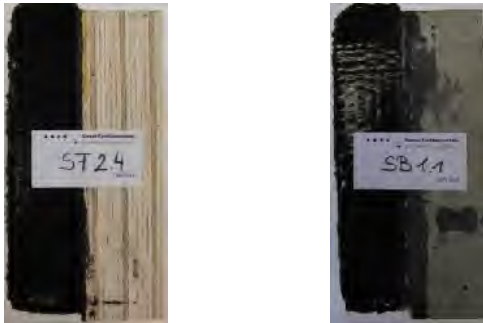
Figure 4: Plastic deformation of a test specimen with PBM sealant on CLT (left) and on concrete (right)
