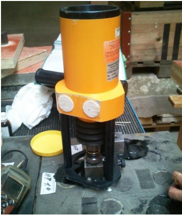
Figure 7: Mobile adhesion tensile testing machine of the company BTS Baucontrol
