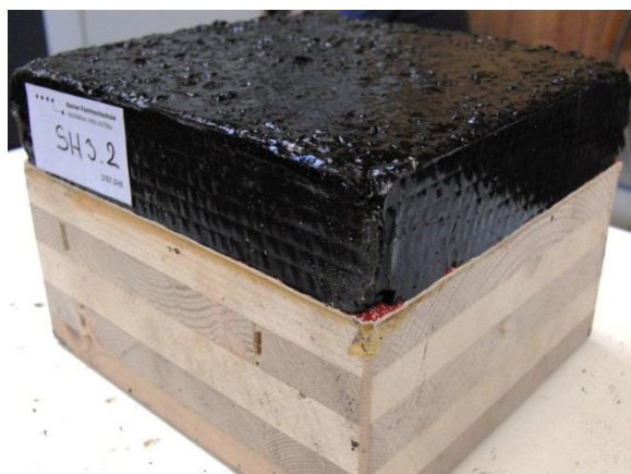
Figure 20: No blistering observed in this specimen of asphalt surfacing on CLT
