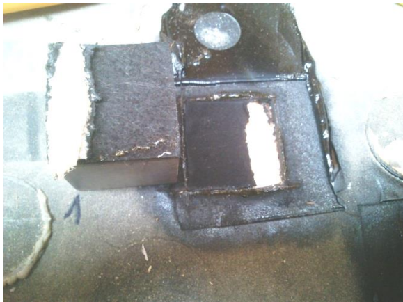
Figure 16: Test specimen with PBM sealant after successful adhesion tensile test [5]
