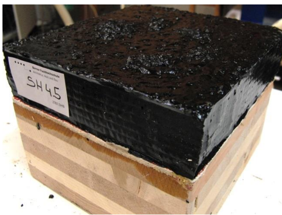
Figure 21: Clear blistering in the surfacing of this specimen of asphalt surfacing on CLT
